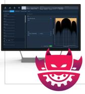
The intuitive SPECTRE UI has two primary modes, Creator and Operational. In Creator mode, the user generates waveforms, power profiles, and band restrictions. In Operational mode the user selects the pre-defined waveforms and profiles to transmit. The system automatically notches any signal that overlaps with restricted bands, allowing users to sweep power onto a system under test.
